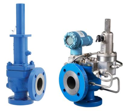
*Figure 4.3: Direct spring load (left) and pilot-operated valves (right) function differently, but* both can leak, making characteristic sounds. Pilot-operated valves can also be diagnosed by monitoring internal pressures.
