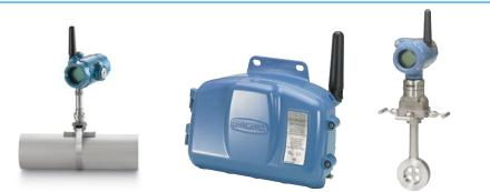
Figure 2.3: Using WirelessHART instruments for heat exchangers simplifies installation. Rosemount X-well™ Technology (left) does not require a thermowell or process penetration. Where conventional temperature sensors are preferred, the Rosemount 848T Wireless Temperature Transmitter (middle) can send data from four sensors via one signal. A Rosemount 3051SFC Wireless Compact Orifice Plate Flow Meter (right) can measure fluid flow in tight spaces.
