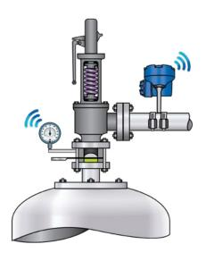
Figure 4.4: Mounting a Rosemount 708 Wireless Acoustic instrument on the discharge pipe of a PRV detects when release incidents happen, and if leakage continues due to an incomplete seal. No process penetration or shutdown is necessary for mounting.
