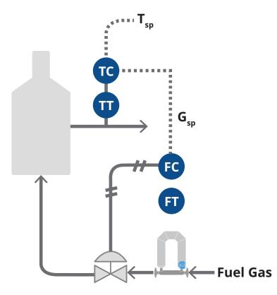
*Figure 1.4: Fuel flow measured in pounds or kilograms* per hour makes it much easier determine optimal stoichiometric air flow.
